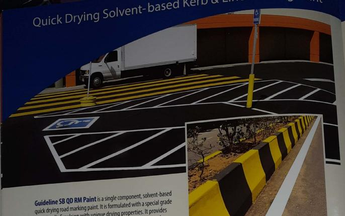
**Guideline SB QD RM Paint** is a single component, solvent-based quick drying road marking paint. It is formulated with a special grade of TP Acrylic Emulsion with unique drying properties. It provides excellent wear and weather resistance thus ensuring road safety. Suitable for application on kerbs, concrete and bituminous road surfaces, it has the unique capability of drying within 15 minutes\*\*.
